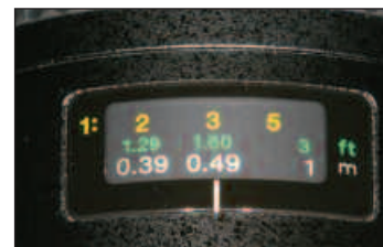
Figure 12. Lens set at 1:3 to provide 1:2 magnification.
